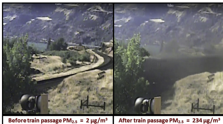
Fig. 3. Images captured from the video camera before and after coal train passage on 8/7/2014 at 17:28 PDT. The full video of this train passage is archived as part of the supplemental materials for this paper. The camera looks to the west, downriver in the Columbia River Gorge. The coal train is visible in the right image and was moving from left to right.
